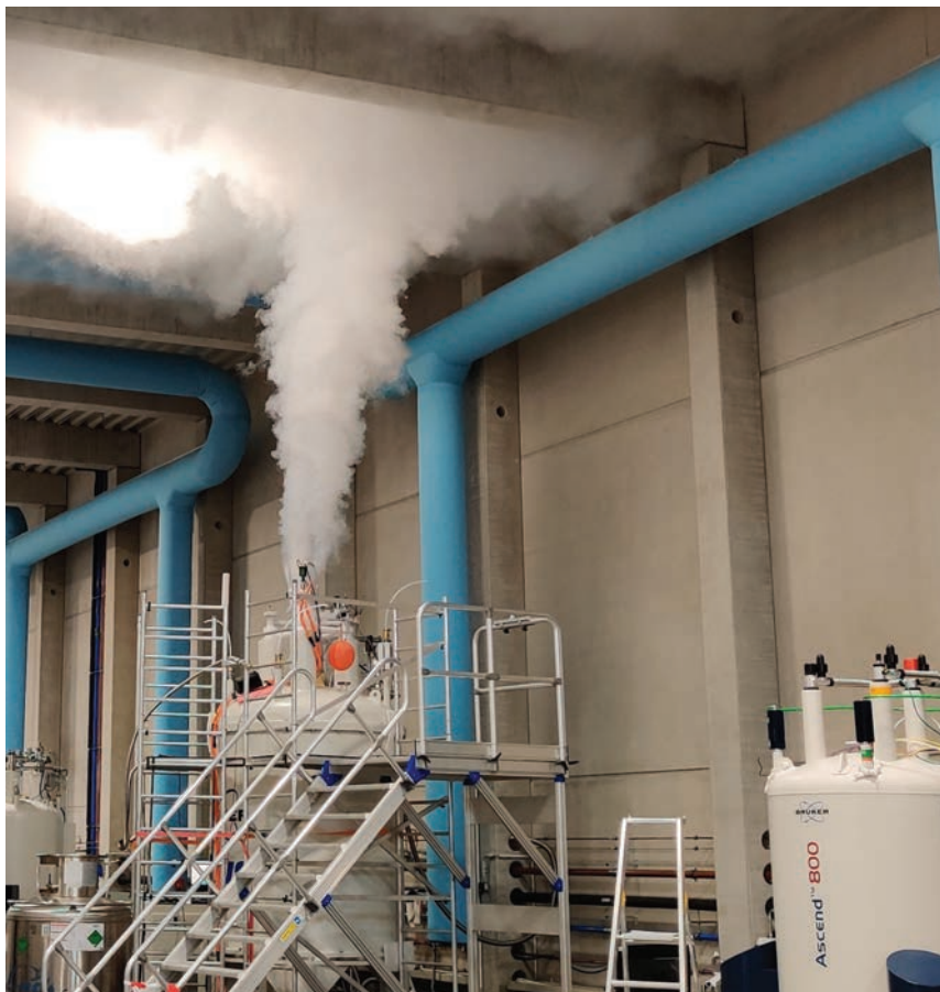
◀ A 22.3-tesla NMR magnet at the Technical University of Munich vents its helium in February 2024 after part of the superconducting coil became resistive. Often, the rate and volume of gas escape in such quenches are too large for recovery systems to handle; in the case shown, the gas could have filled a small blimp. (Photo courtesy of Matthias Brandl.)
