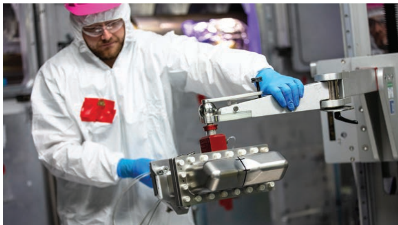
▲ Inside the metal case shown here are weapons-grade plutonium samples. To better understand the effect that a hostile environment, such as a missile defense system, may have on US nuclear weapons, researchers at the National Ignition Facility exposed the plutonium to intense pulses of neutrons in 2025. The radiation was generated by the implosion and heating of nuclear fusion fuel by incident lasers. (Photo by Jason Laurea/LLNL.)
