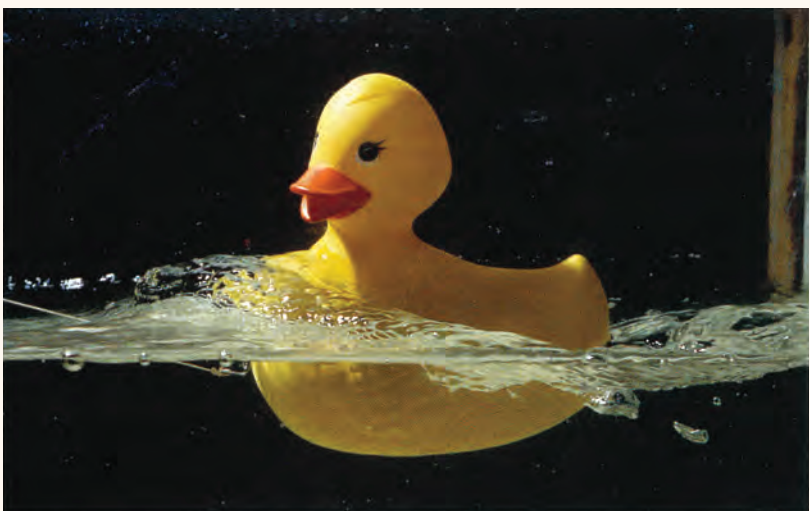
◀ Figure 1. Rubber ducky being towed in a flow tank just under ( top ) and just over ( bottom ) its hull speed. Notice that at the higher speed this small surface ship tips upward and its stern wave disappears.
