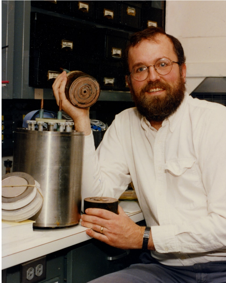
Figure 3: One of world-record 72T pulsed magnets [18], shown with the author holding two halves of a second magnet coil (cut in half to facilitate post-pulse analysis). The experimental sample and plastic cryostat tails fit inside the 9.2mm diameter clear bore of the magnet coil at the center of the coil windings. At extreme left is one of the twelve thyristors used to switch the capacitor bank that energized the magnets. The thyristors were stacked three in series and four in parallel to handle the 12kV voltage and 325kA current specifications, respectively.
