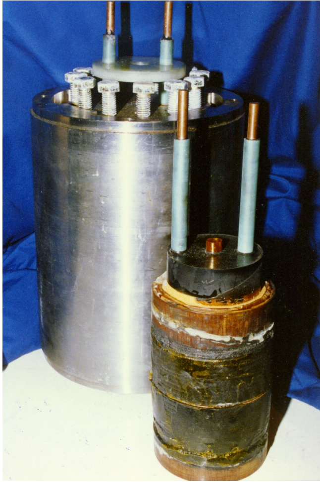
Figure 2: The two world-record 72T pulsed magnets [18]. At left is the completely assembled magnet, housed in the VascoMax steel casing used to precompress the magnet coil... and to contain any “magnet disassembly events”. At right is the magnet coil removed from its casing, wound with three different conductors chosen for high ductility (layer 1), high strength (layers 2-7), and high conductivity (layers 8-14).
