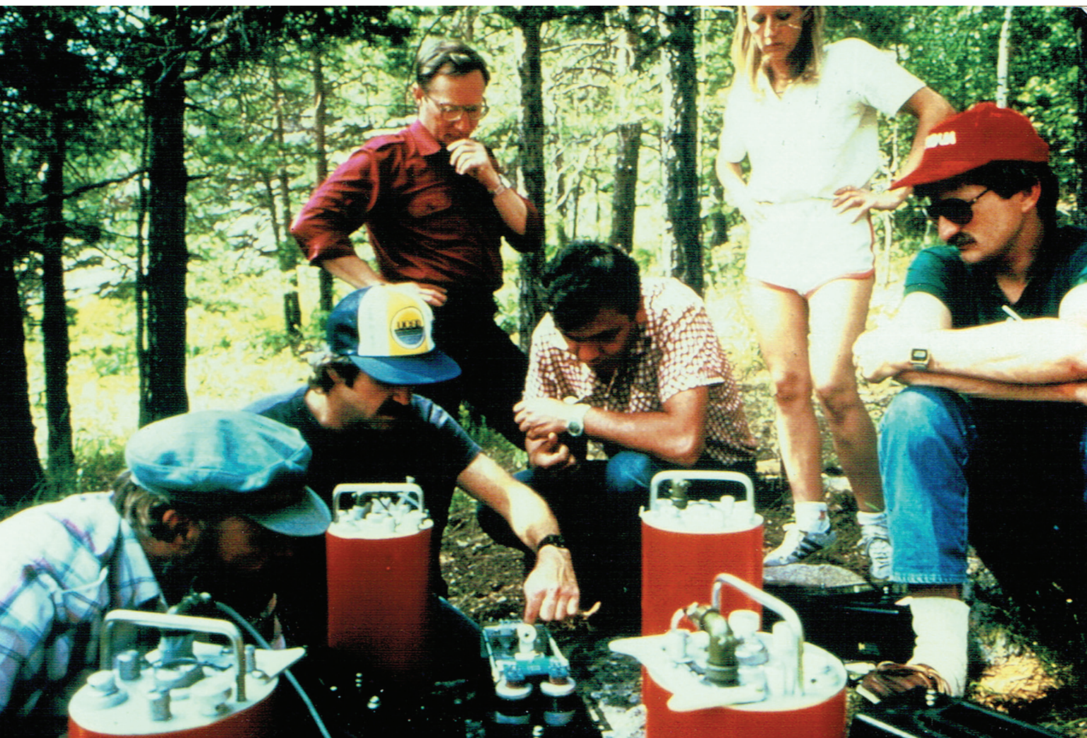
▲ US seismologists with seismometers on a granite outcrop about 200 kilometers from the Semipalatinsk Test Site in northeastern Kazakhstan to measure surface background noise. Permanent seismometers were placed in 100-meter-deep boreholes to isolate them from the surface noise.
