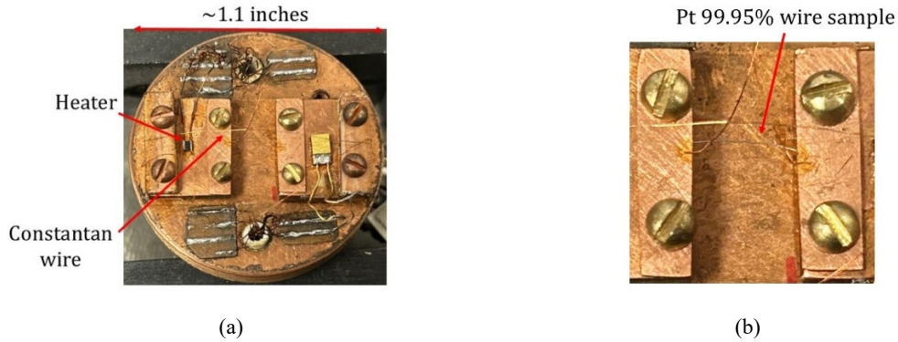
FIGURE 2. (a) Top view of a thermopower probe with the hot platform on the left and the cold platform on the right. (b) Close-up view of a thermopower probe focused on the 99.95% Pt wire sample suspended across the platforms.
