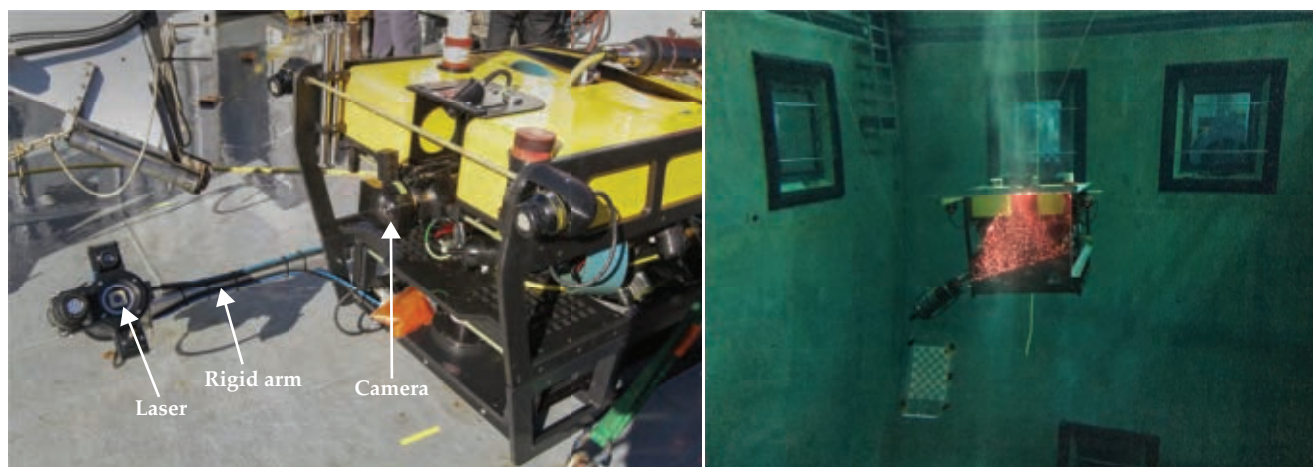
FIGURE 2. TETHERED to a ship on the ocean surface, (a) this remotely operated vehicle (ROV) controls the position of the DeepPIV instrument mounted to its frame. Using the ROV camera and a laser extended by a half-meter rigid arm, the instrument collects video data for particle velocimetry experiments and three-dimensional reconstructions. The laser projects a sheet of light that illuminates the motion of suspended particles and the interior structure of any sea creature nearby. The camera captures the lit objects. (b) Extending from the ROV, the laser illuminates air bubbles in a laboratory tank. (Courtesy of MBARI.)
