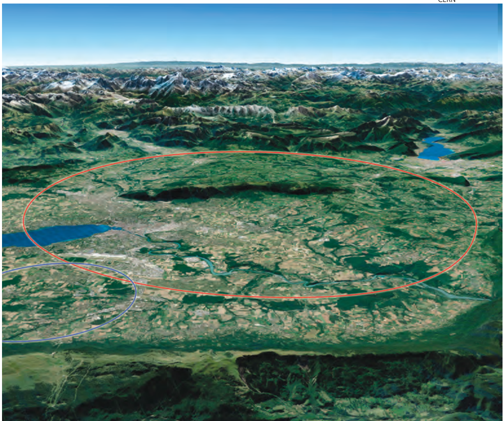
THE 100-KM-CIRCUMFERENCE FUTURE CIRCULAR COLLIDER (orange circle) would pass beneath Lake Geneva. It could start out as an electron-positron collider and be upgraded to a 100 TeV hadron collider. A feasibility study on whether to go ahead with it is a top priority in the 2020 European Strategy for Particle Physics. The blue circle shows the position of the Large Hadron Collider.
