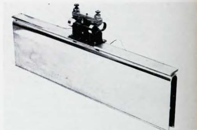
Fig. 3. Aluminum tuning fork ( \frac{1}{4} scale model of dimensions 50 \times 13.5 \times 3.5 cm).
