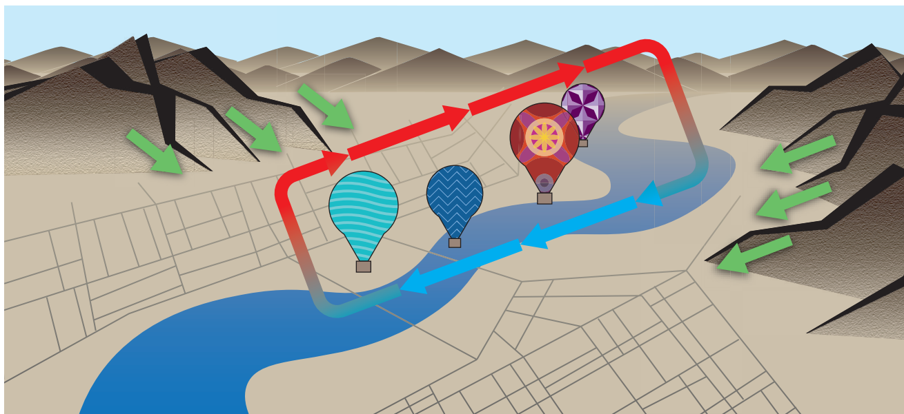
FIGURE 2. THE ALBUQUERQUE BOX is a unique wind circulation in and around the city. When cold, dense air (green arrows) flows from the surrounding mountainous terrain toward the Rio Grande, a northerly drainage wind (blue arrows) develops and moves from higher elevation in the north to lower elevation in the south. In the river valley, temperature increases with altitude, which is called a temperature inversion. Above the inversion, the large-scale wind pattern dictates the box wind's direction. For the Albuquerque box, the large-scale wind (red arrows) travels from south to north. (Image by Freddie Pagani.)
