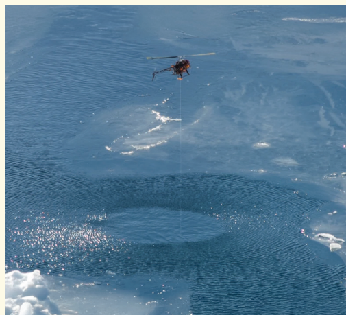
FIGURE 1. AN UNCREWED HELICOPTER hovers over Sermilik Fjord in March 2023 as a sensor that was lowered under the surface collects data. (Image adapted from K. Hansen et al., Nat. Geosci. 18 , 219, 2025.)
