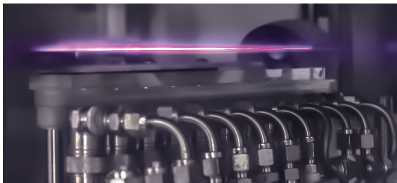
FIGURE 2. A PLASMA CHANNEL , 30 cm long, acts as a conduit for a laser pulse used to create a plasma wakefield that accelerates electrons to high energies at the Berkeley Lab Laser Accelerator Center. The plasma is formed when a 40 fs laser pulse is shot through a sheet of supersonic gas that streams upward out of an aluminum slit. The pink color is a result of the hydrogen gas used to generate the channel. (Photo courtesy of Alex Picksley and Anthony Gonsalves, Lawrence Berkeley National Laboratory.)
