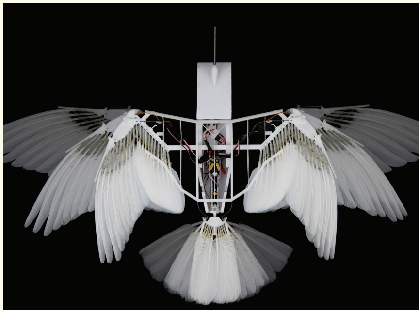
DESIGNED TO FLY LIKE A BIRD , PigeonBot II doesn't rely on a rudder to prevent rolling and yawing. Instead, the wings and tail can shift into multiple positions in response to turbulence. (Image courtesy of Eric Chang, Lentink Lab.)
