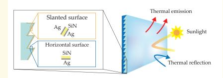
**TO COOL A WALL**, a material must emit IR radiation toward the sky while reflecting the radiation coming at it from the ground. It can do that with a sawtooth pattern of facets, with the upward-facing surfaces made of IR-emitting silicon nitride and the downward-facing surfaces made of highly reflective silver. (Figure adapted from F. Xie et al., *Science* **386**, 788, 2024.)
