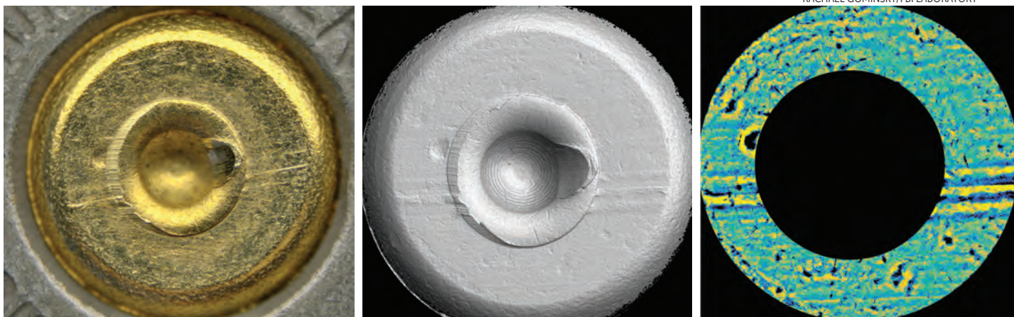
ANALYSIS FROM THIS CARTRIDGE CASE (left), shot with a 9 mm Luger pistol, is part of a database that the FBI, NIST, and the Netherlands Forensic Institute are working on to help assign a likelihood to whether a bullet or casing was fired by a given gun. The features that would catch an examiner's attention are the lines, the firing pin impression at the center, the drag at 3 o'clock, and the crescent-shaped toolmark running around the firing pin from 7 to 11 o'clock. The center image shows a scan of the cartridge case, which is used to obtain the coordinates of toolmarks. The right-hand image is a map of the depths of the toolmarks made with focus variation scanning; black represents deep spots and yellow represents high spots.
