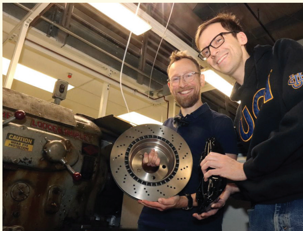
UNIVERSITY OF CALIFORNIA RESEARCHERS Paulus Bauer (left) holds a brake rotor and Adam Thomas holds a brake caliper next to the lathe that they and their colleagues used to simulate automotive brake emissions. (Courtesy of Lucas Van Wyk Joel, University of California, Irvine.)
