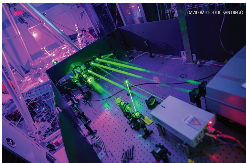
LASER INTERFEROMETRY is used to probe the density and other properties of deuterium plasmas in Farhat Beg's lab at the University of California, San Diego. The lab now works with the university's Fusion Engineering Institute.
