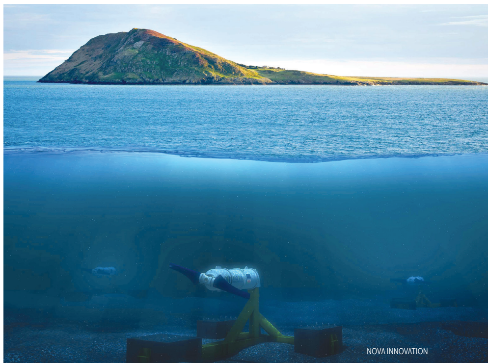
ROWS OF TURBINES in the currents generated by the rise and fall of the tides offer a predictable way of producing electricity. Here, an array of 100 kW turbines sits on the Bluemull Sound seafloor off Scotland's Shetland Islands.
