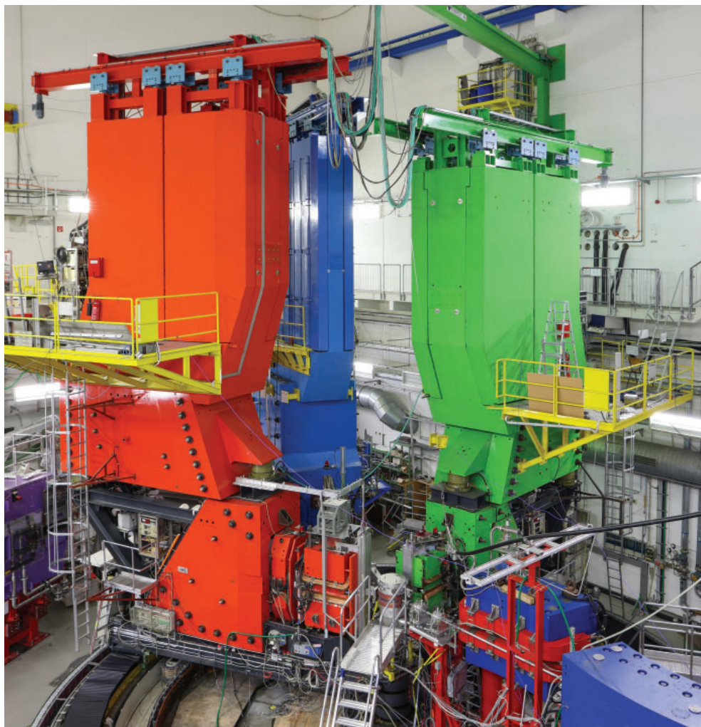
FIGURE 1. THE MAINZ MICROTRON , a particle accelerator at the Johannes Gutenberg University Mainz in Germany, includes this experimental hall that features a trio of high-precision spectrometers in red, blue, and green. The setup recently provided improved electron-scattering measurements of the alpha particle's cross section when in its excited state. Those results disagree with theoretical calculations, which opens questions for the nuclear-physics community. (Photo by Alexander Sell, JGU.)
