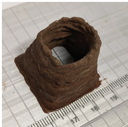
HUMAN BEINGS naturally produce serum albumin and urea. The first can be extracted from their blood plasma, and the second from their urine, sweat, and tears. Combined with Martian regolith, those ingredients can make a biocomposite material termed AstroCrete—pictured as a 3D-printed structure ( left ) and a brick ( right )—that's stronger than terrestrial concrete.
