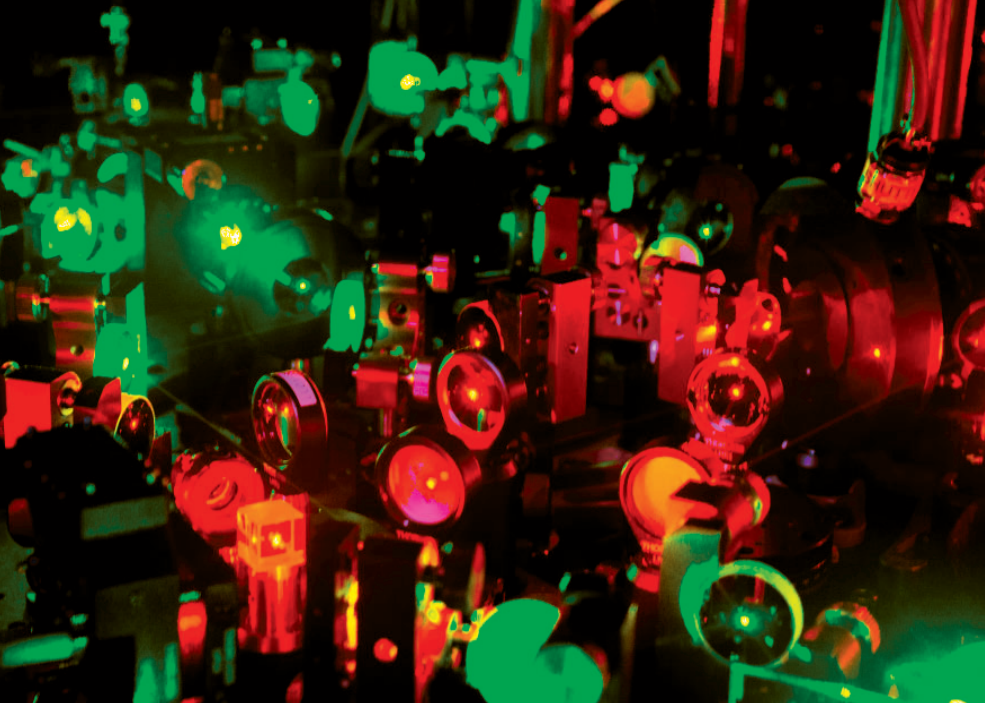
FIGURE 1. A THICKET of optical elements directs the laser beams that cool and trap the triatomic molecule calcium monohydroxide. Laser cooling and magneto-optical trapping of atoms is standard practice, and a few groups have succeeded in cooling and trapping diatomic molecules. But never before has a three-atom molecule received the same treatment. (Photo by Loïc Anderegg.)
