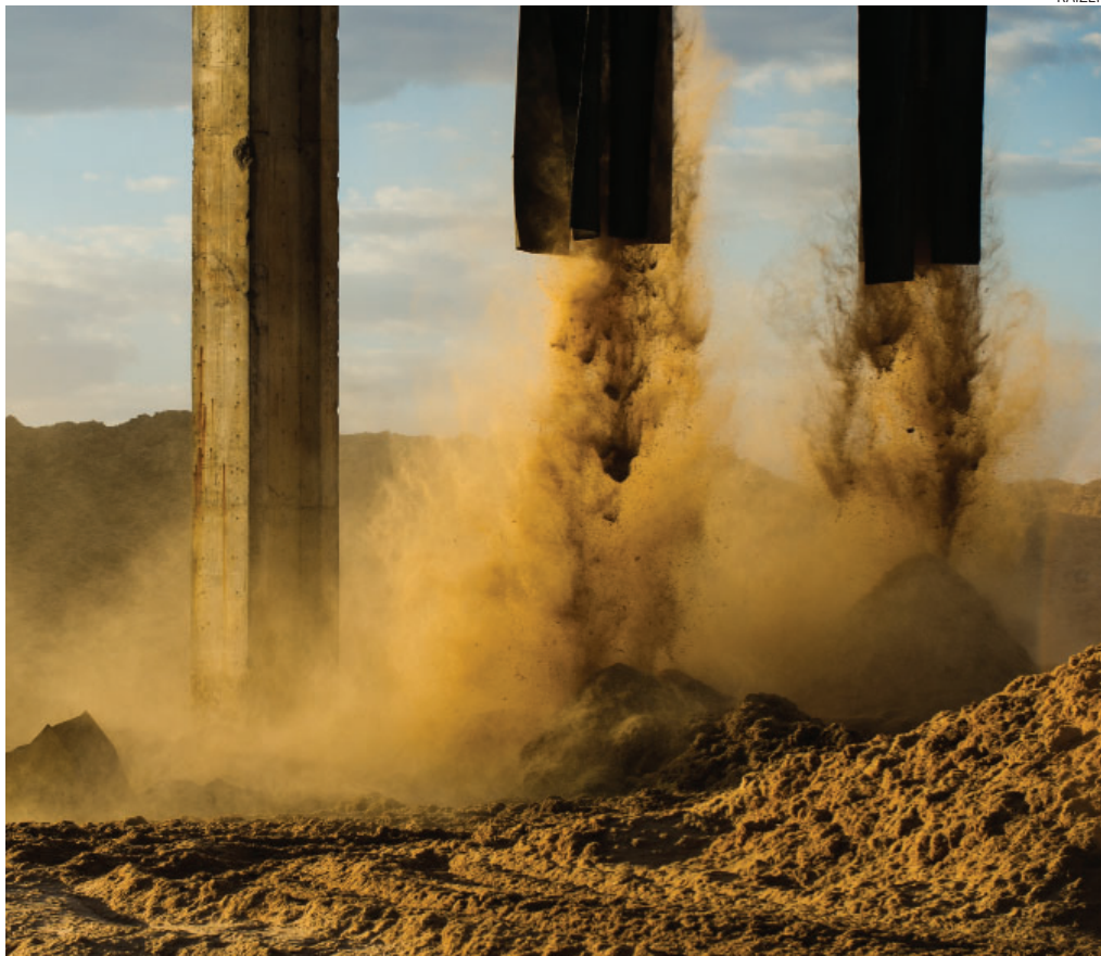
RAÍZEN'S PLANT in Piracicaba, Brazil, is the world's only commercial producer of cellulosic ethanol. Here, crushed sugarcane residue called bagasse is being loaded into the processing plant. Raízen plans to build 20 such plants by 2030.
