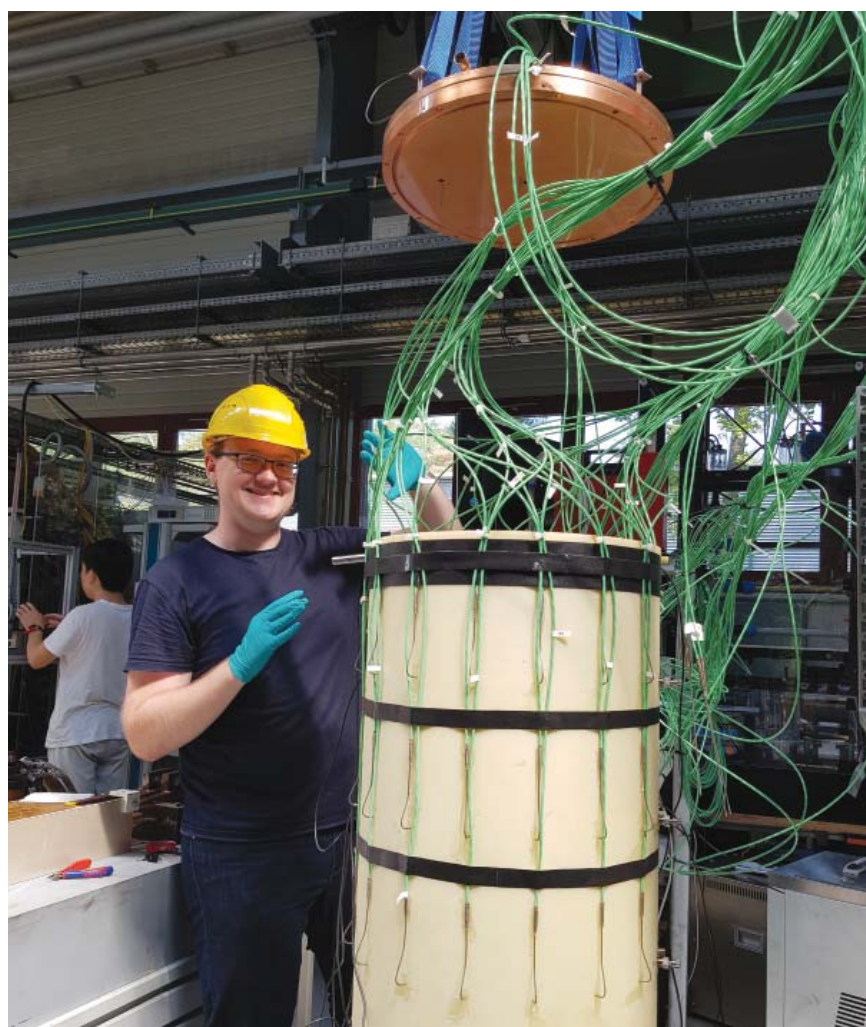
FIGURE 1. FELIX SCHINDLER, a PhD student at the Helmholtz-Zentrum Dresden-Rossendorf, assembles a cylindrical drum to be filled with liquid metal for turbulent convection experiments. (Photo by Tobias Vogt.)
