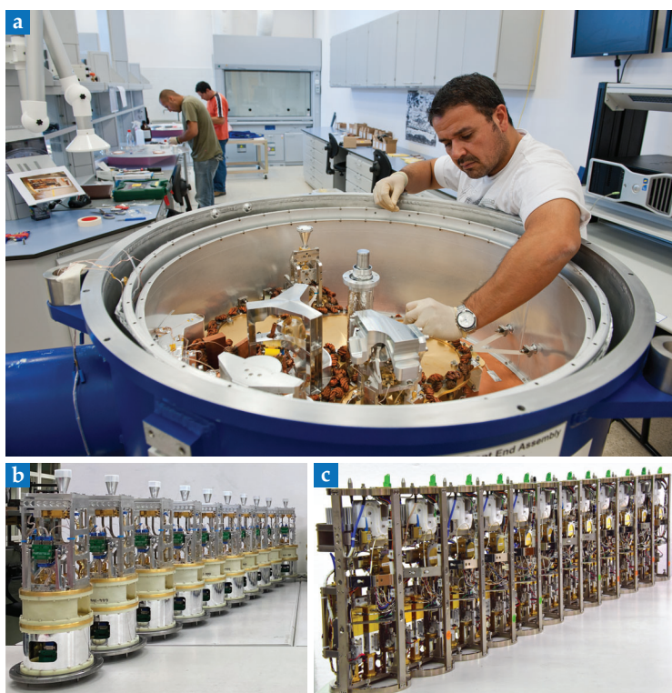
FIGURE 4. ANTENNA COMPONENTS used in the Atacama Large Millimeter/Submillimeter Array (ALMA) telescope include (a) a cryostat, here being assembled by technician Patricio Escarate. It cools 10 receiver cartridges. The (b) cold receiver cartridges are paired with (c) warm receiver cartridges. Together, the assemblies are used to make observations in the 35–50 GHz frequency range. (Panel a courtesy of ESO/Max Alexander; panel b courtesy of ASIAA; and panel c courtesy of G. Siringo, ALMA, ESO/NAOJ/NRAO.)
