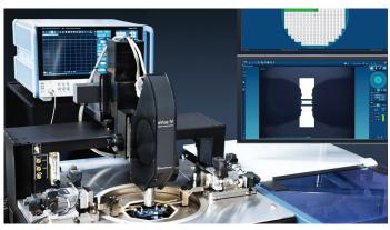
probe systems including high-frequency probes, probe positioners, and thermal control and calibration tools. FormFactor WinCal XE software calibrates the complete test system, including the R&S ZNA. *Rohde & Schwarz GmbH & Co KG*, *Mühldorfstraβe* 15, 81671 *Munich, Germany, www.rohde-schwarz.com*
