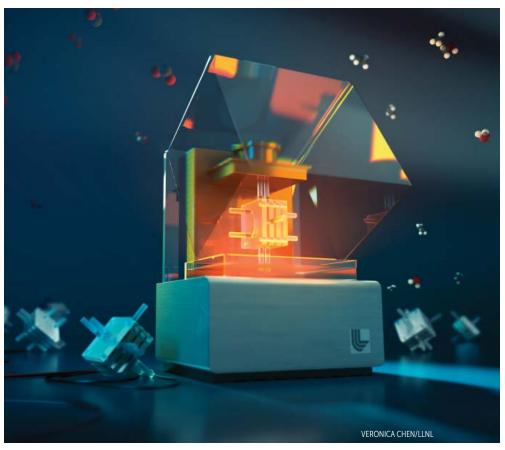
**THREE-DIMENSIONAL PRINTING** can shorten the time it takes to make improved versions of devices to electrochemically convert carbon dioxide to chemicals. Shown here is a rendition of a 3D printer with a palm-sized reactor housing being printed. Assembled reactors are on the table. The research is a collaboration between Stanford University, the oil and gas company Total American Services, and Lawrence Livermore National Laboratory.
