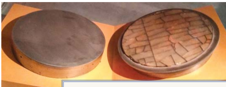
FIGURE 3. A RESONANT QUARTZ SANDWICH TRANSDUCER previously owned by the French Navy. The instrument, which has a diameter of 10 cm, is now on display at the ESPCI Paris. It has been opened to show the quartz mosaic attached to the quarter-wave steel plate on the right.
