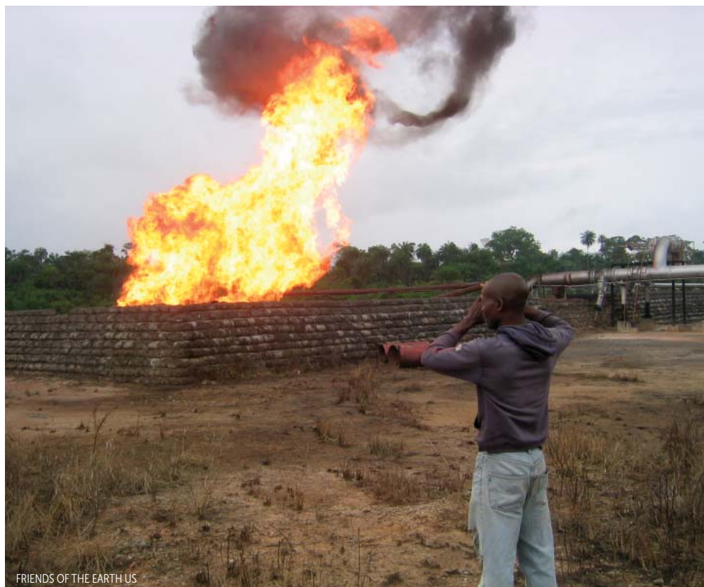
GAS FLARES , like this one in Nigeria, burn methane to safely depressurize oil wells, but they also release toxic gases and particulates and contribute to global warming.
