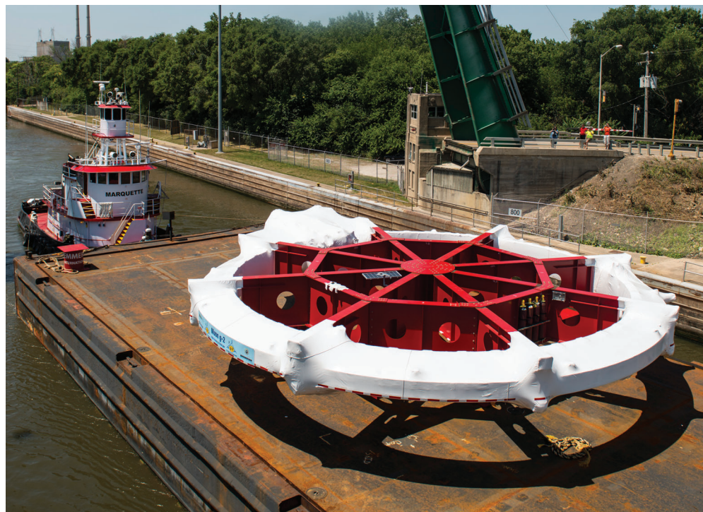
FIGURE 1. THE MAGNET RING for Fermilab's Muon g - 2 experiment measures an unwieldy 14.2 meters across. It traveled by barge and on special trucks during its relocation to Illinois from Brookhaven National Laboratory in New York. (Courtesy of Reidar Hahn/Fermilab.)
