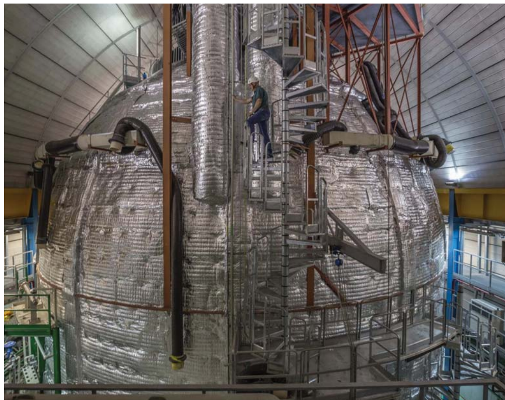
FIGURE 1. THE BOREXINO NEUTRINO DETECTOR , after being wrapped in an aluminum-reinforced wool blanket in 2014 and after the installation of a temperature control system in 2019. Solar neutrinos are detected in its inner 8.5-meter-wide balloon filled with 280 tons of petroleum-based scintillator liquid. The scintillator emits flashes of light when the neutrinos scatter from its electrons. 2
