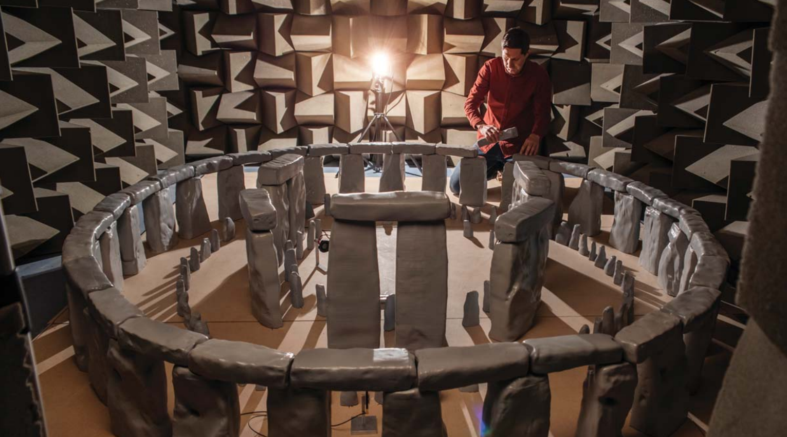
THIS ACOUSTIC SCALE MODEL of Stonehenge is housed in a semi-anechoic chamber at the University of Salford in the UK. At 2.5 m wide, the model mimics the monument circa 2200 BC, when it had 157 stones. Today's ruin contains roughly half that number. The light is at sunrise for the midsummer solstice. Foam wedges on the chamber's walls mimic the sound absorption in the open countryside surrounding the real site. (Author Trevor Cox is seen behind the model.)
