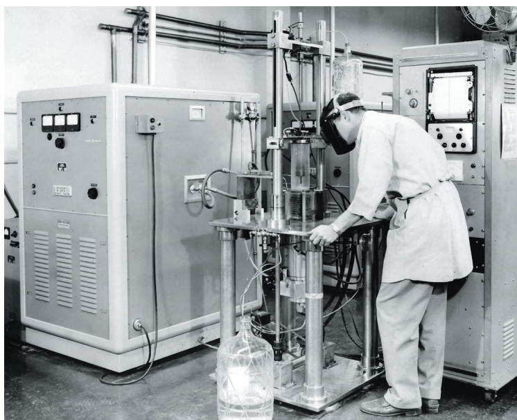
FIGURE 2. KNAPIC ELECTRO-PHYSICS was one of the first companies to sell silicon crystals. It produced them using the Czochralski method, which required machinery like the crystal puller pictured here. (Courtesy of the Arthur del Prado Collection.)
