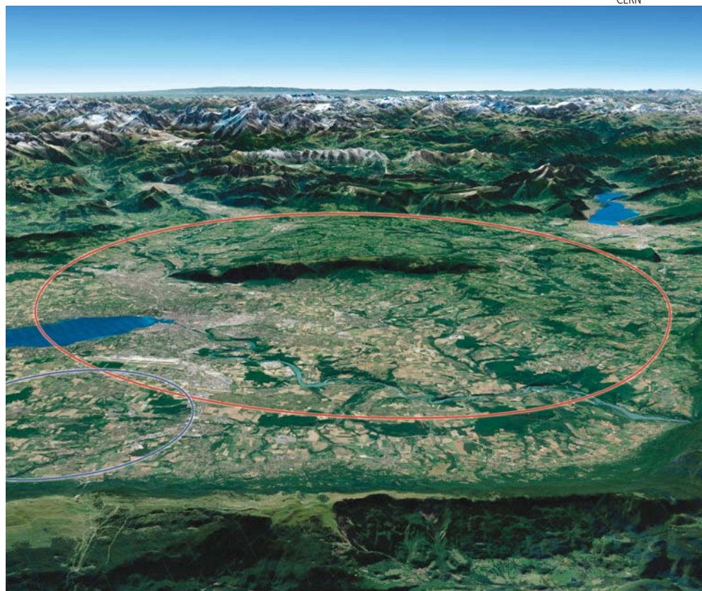
THE 100-KM-CIRCUMFERENCE FUTURE CIRCULAR COLLIDER (orange circle) would pass beneath Lake Geneva. It could start out as an electron-positron collider and be upgraded to a 100 TeV hadron collider. A feasibility study on whether to go ahead with it is a top priority in the 2020 European Strategy for Particle Physics. The blue circle shows the position of the Large Hadron Collider.
