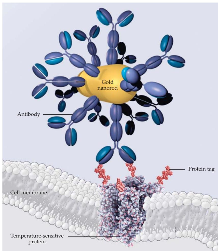
**FIGURE 1. HOW TO SEE IN THE NEAR-IR.** A gold nanorod strongly absorbs 915 nm light to produce heat, and a temperature-sensitive protein generates an electrical signal when heated. When the protein is embedded in a retinal cell membrane and linked to the nanoparticle via a protein tag and corresponding antibody, the retina becomes sensitive to near-IR light that most animals can't normally see. (Image by Veronique Juvin, SciArtWork.)
