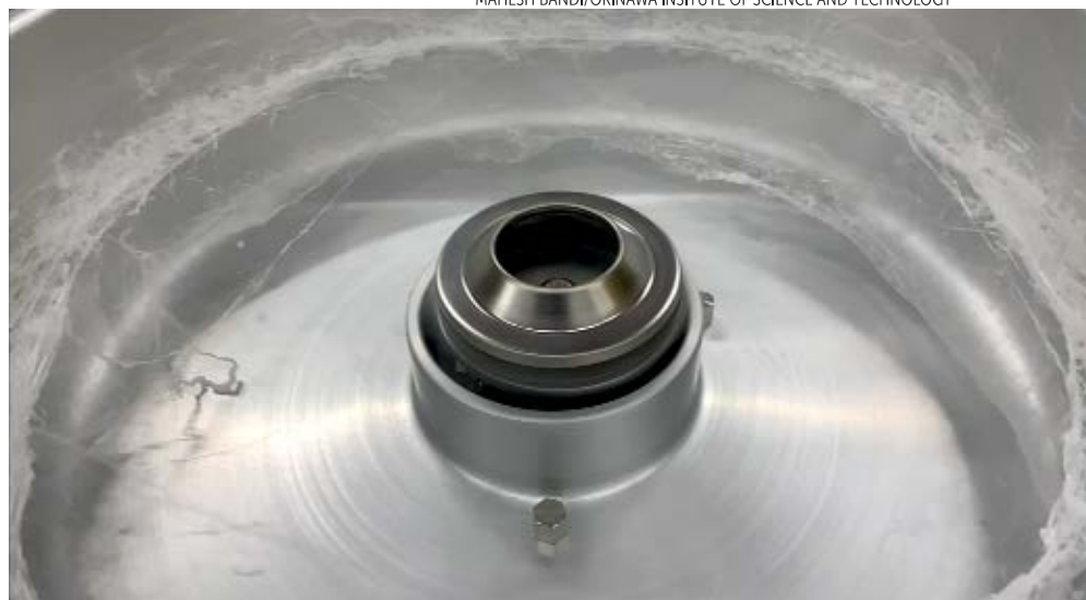
THIS COTTON CANDY MACHINE (diameter 70 cm) was retooled to make a high-quality filter material for face masks. The technique could enable inexpensive, local fabrication, especially in less developed regions of the world.
