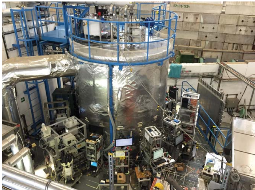
FIGURE 3. THE CLOUD (COSMICS LEAVING OUTDOOR DROPLETS) CHAMBER at CERN is a 26-cubic-meter tank in which temperature and gas concentrations are carefully controlled to simulate natural atmospheric conditions between the ground level and the stratosphere. The proton synchrotron serves as an artificial source of cosmic rays, which simulates natural atmospheric conditions and may stabilize particles that form from the ionized gases in the chamber. External instrumentation allows for constant monitoring of the chamber's contents. (Courtesy of CERN/Neil Donahue.)
