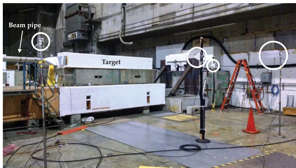
FIGURE 2. THE EXPERIMENT AT SLAC. Electrons exit the beam pipe (far left) and enter the 4-m-long polyethylene target, surrounded by transmitter and receiver antennas (circled). Second from left is the transmitter; the others are receivers. (Adapted from ref. 5.)
