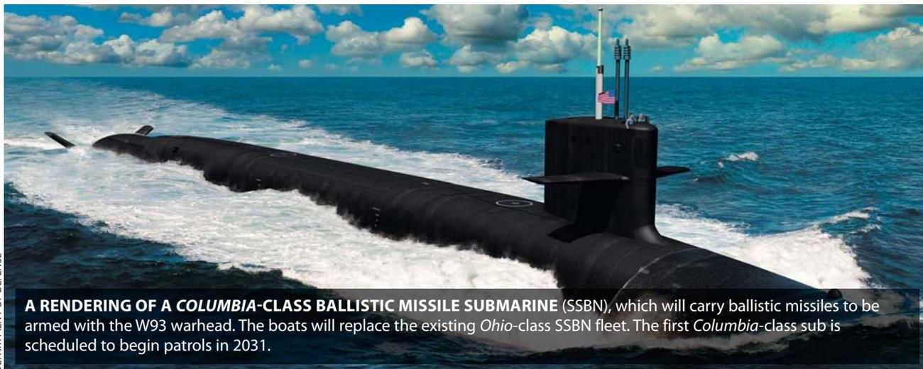
**A RENDERING OF A COLUMBIA-CLASS BALLISTIC MISSILE SUBMARINE (SSBN)**, which will carry ballistic missiles to be armed with the W93 warhead. The boats will replace the existing *Ohio*-class SSBN fleet. The first *Columbia*-class sub is scheduled to begin patrols in 2031.
