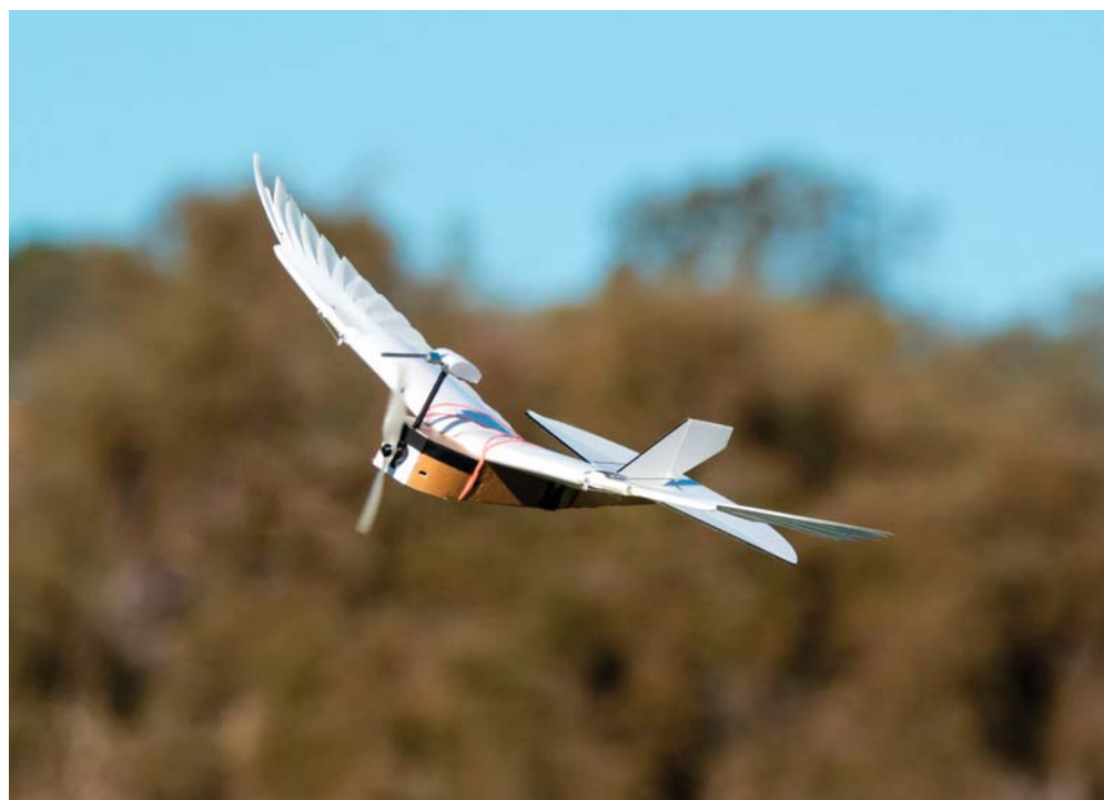
FIGURE 1. THIS BIOHYBRID ROBOT combines mechanical parts with pigeon feathers. During real-world flight tests with high and low turbulence, PigeonBot controlled the position of its 40 feathers using four wing-mounted motors. The feathers’ fasteners prevented any gaps in the wings from forming that would have otherwise limited the robot’s mobility. (Lentink Lab/Stanford University.)
