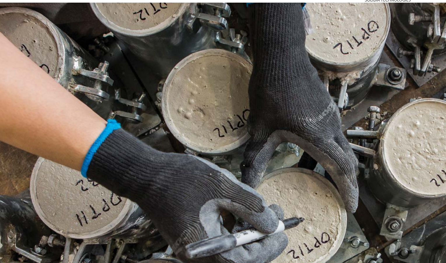
SAMPLES OF NOVEL CONCRETE in cylinders are tested by Solidia Technologies employees prior to curing with CO 2 . Building materials present a route to permanently remove CO 2 from the atmosphere.
