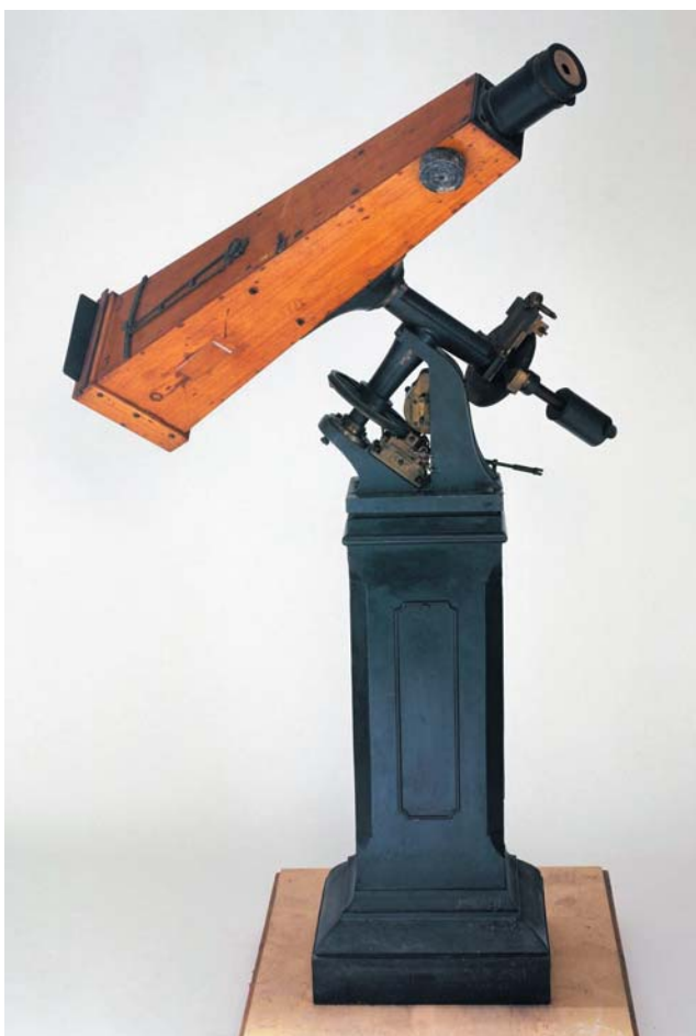
FIGURE 1. THE KEW PHOTOHELIOGRAPH , an instrument that combined a telescope with a camera for eclipse observation and photography, designed by Warren De la Rue. (Courtesy of the Science Museum Group Collection, CC BY 4.0.)
