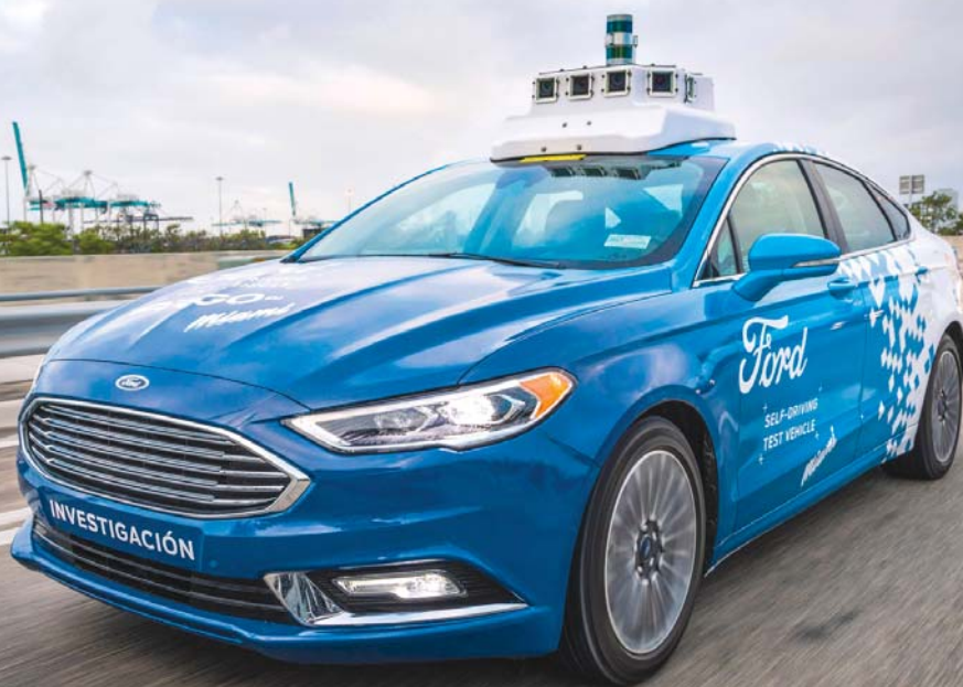
A FORD ARGO VEHICLE in action. Visible on the roof are two lidar units (top) and multiple video cameras (bottom).
