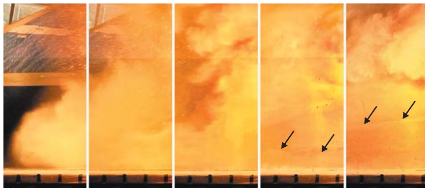
FIGURE 1. THE VOLCANO ERUPTION SIMULATOR FACILITY at Massey University in New Zealand produces experimental pyroclastic flows—hot avalanches composed of air, ash, and rock—that allow the study of their dynamical behavior. In this series of images spanning about a second, the bottom meter of a two-layer flow passes a fixed observation point. The arrows denote the boundary between a denser particle layer overridden by dilute, turbulent ash.
