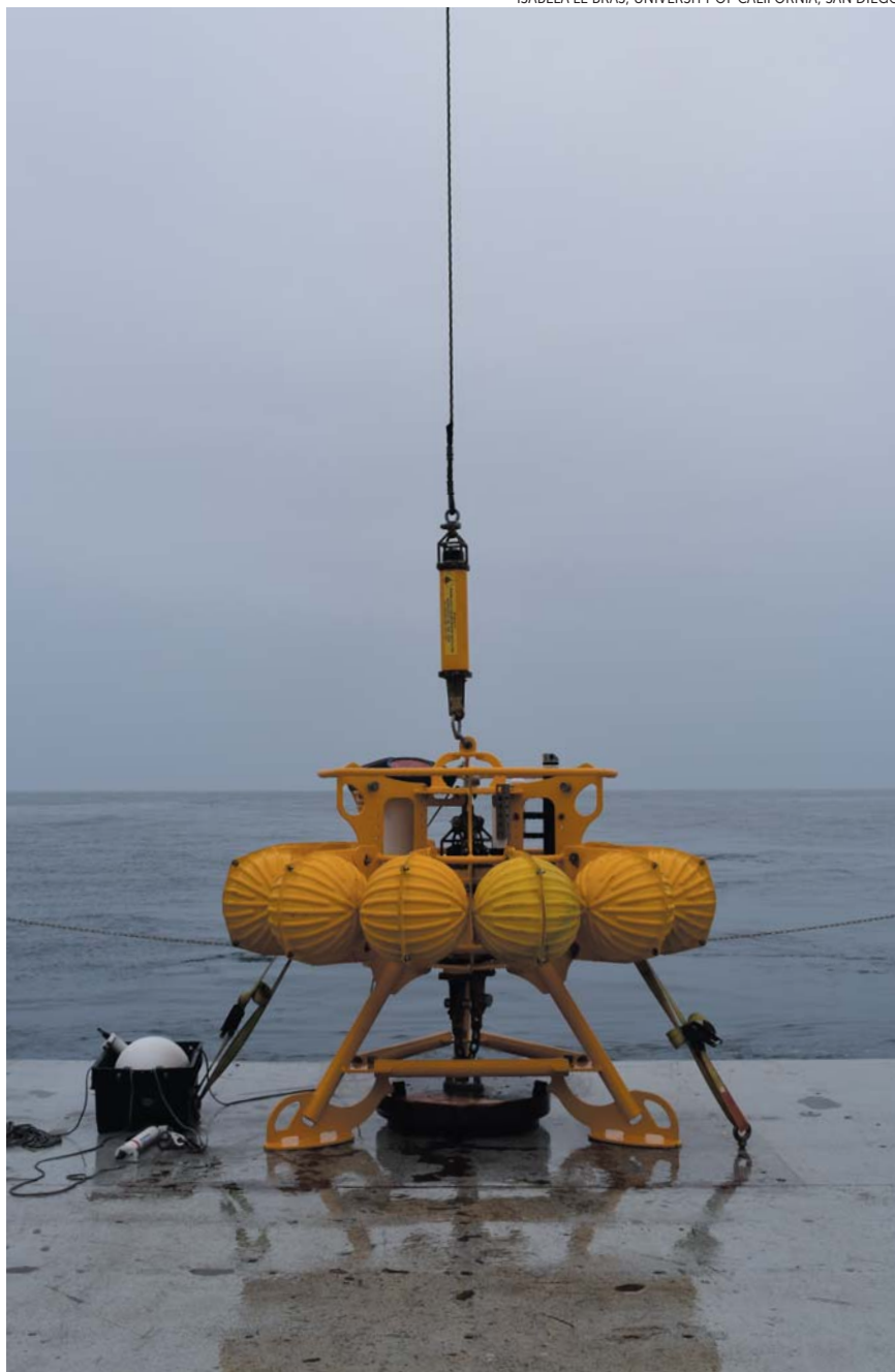
FIGURE 2. THE MOORING SHOWN HERE will sit on Greenland's continental shelf 200 m below the surface. While the yellow portion anchors the mooring to the seafloor, the instruments in the black box to the left float above it and collect continuous measurements of temperature, salinity, and velocity at multiple depths.
