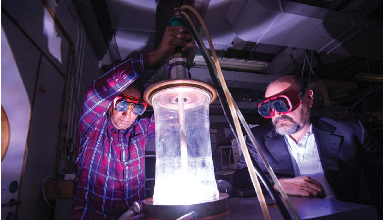
STEFANO SANVITO (RIGHT) AND MUNUSWAMY VENKATESAN of Trinity College Dublin melt metallic powders to create new magnetic compounds. Sanvito's team uses computer simulations to design magnetic materials and has created many of them.
