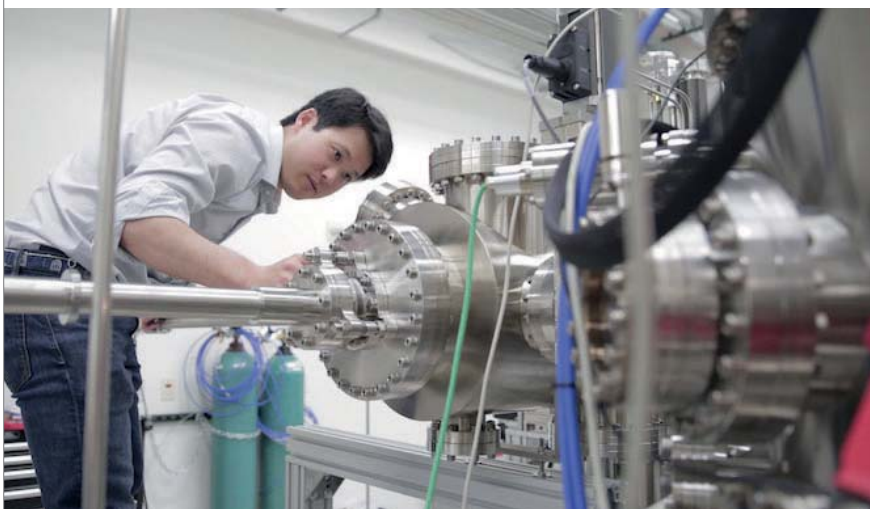
Jason Kawasaki transfers a sample into the molecular beam epitaxy system for film growth. Photo credit: University of Wisconsin-Madison, College of Engineering External Relations.
