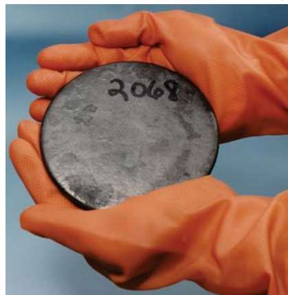
A "BUTTON" OF HIGHLY ENRICHED URANIUM metal. HEU comes in various forms, including oxides, solutions, and new or irradiated reactor fuel. All HEU is considered weapons usable.
