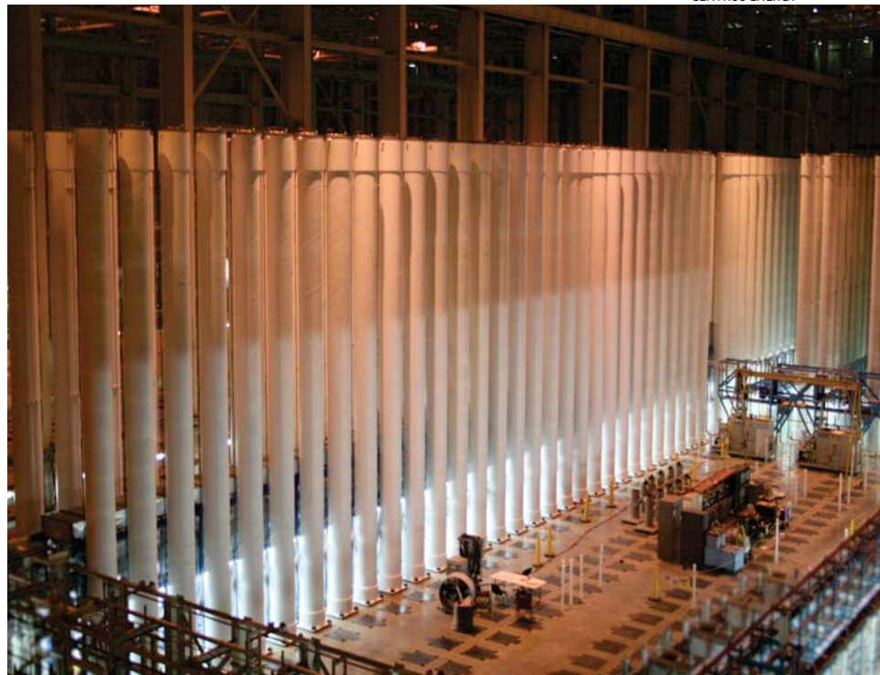
A CASCADE OF AC100 CENTRIFUGES was operated for three years in a technology demonstration at a Centrus Energy facility in Piketon, Ohio.
