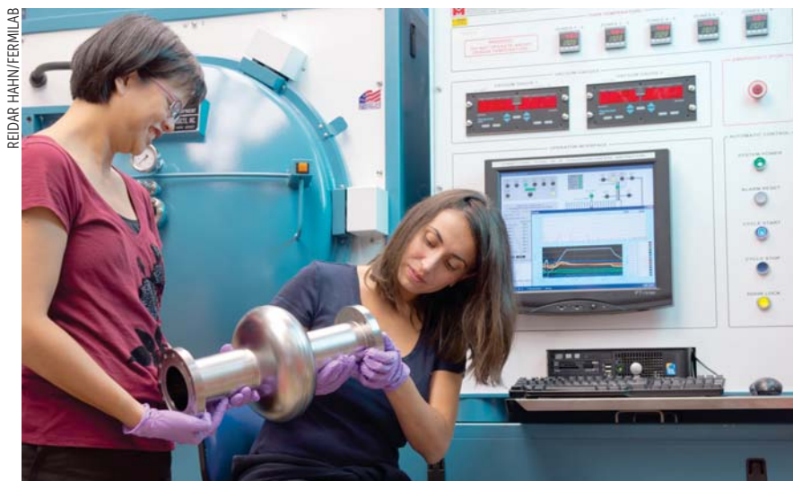
FERMILAB'S ANNA GRASSELLINO (right) and Mayling Wong-Squires study how nitrogen doping and infusion increase the performance of superconducting RF cavities such as those the International Linear Collider would use. They are readying a cavity for baking in the high-temperature oven behind them.
