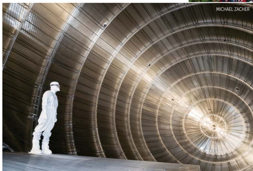
TRANSPORTING THE SPECTROMETER for the Karlsruhe Tritium Neutrino Experiment was a difficult task and a spectacle. Its size required a detour that took it 8400 km, mostly over water, to travel to its destination just 400 km from where it was assembled. Inset: The inside of the 1400-cubic-meter spectrometer.
