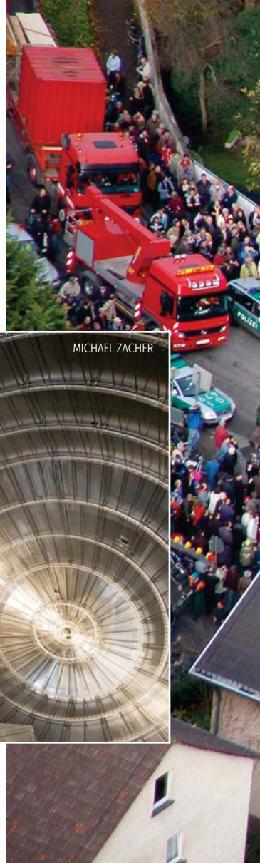
TRANSPORTING THE SPECTROMETER for the Karlsruhe Tritium Neutrino Experiment was a difficult task and a spectacle. Its size required a detour that took it 8400 km, mostly over water, to travel to its destination just 400 km from where it was assembled. Inset: The inside of the 1400-cubic-meter spectrometer.
