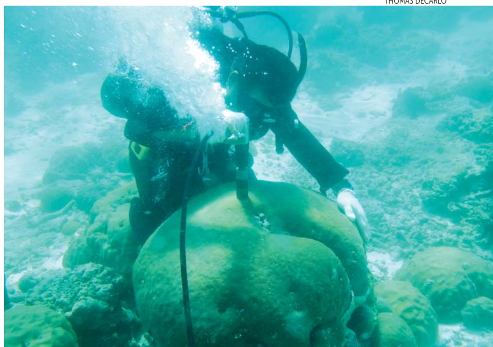
FIGURE 1. TO COLLECT A CYLINDRICAL CORAL SAMPLE , 3 cm across and tens of centimeters long, Kan-Min of the Dongsha Atoll Research Station drills into a large coral colony. The pneumatic drill is powered by a spare scuba tank.
