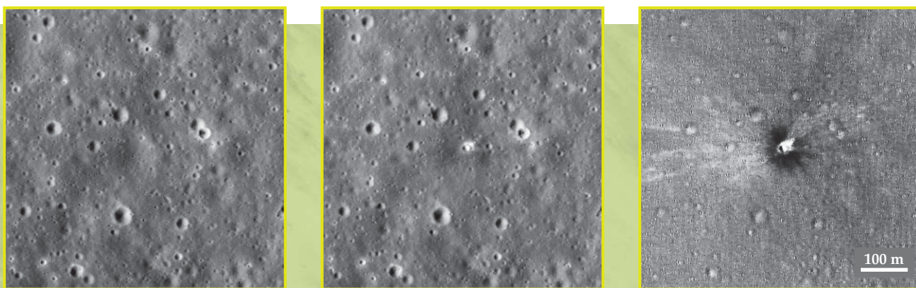
FIGURE 3. A RECENT METEOROID IMPACT was identified by comparing a “before” image from 2012 (left) with an “after” image taken under identical lighting conditions in 2013 (center). The ratio of the two images (right) clearly shows an 11 m crater. Immediately surrounding the crater are areas of high and low reflectance and faint rays that stretch farther out. The landscape changes are due to the deposition of ejecta and to the churning of the soil by impact debris. (Images from the Lunar Reconnaissance Orbiter Camera.)
